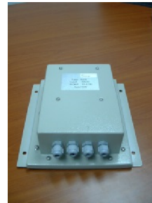
Converter in IP55 enclosure
