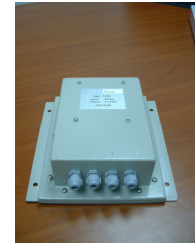
Converter in IP54 enclosure
