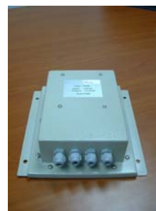
Conveter in IP54 enclosure
